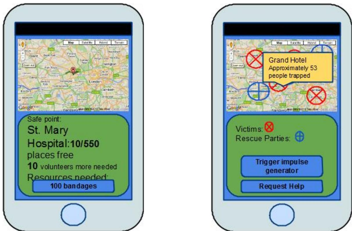
The survival mode switches all other applications off to prolong the battery life for as long as needed, sending only periodical messages. This would allow the server to access their location and provide it to rescue teams in proximity. In survival mode all other connections are turned off, but if triggered by a rescuer's phone nearby, it starts ringing.
